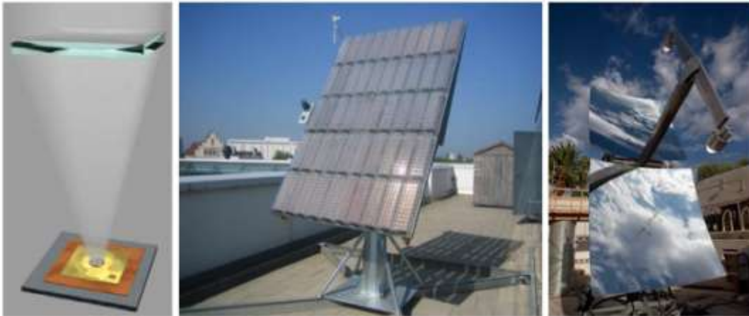
Figure 12. Left and middle: CPV Using Fresnel lenses Right: Mirror-Based.
